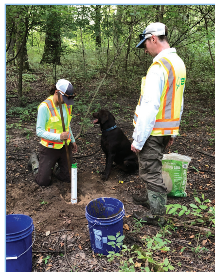
Crew members install groundwater monitoring wells to measure the future positive impact of mitigation.
